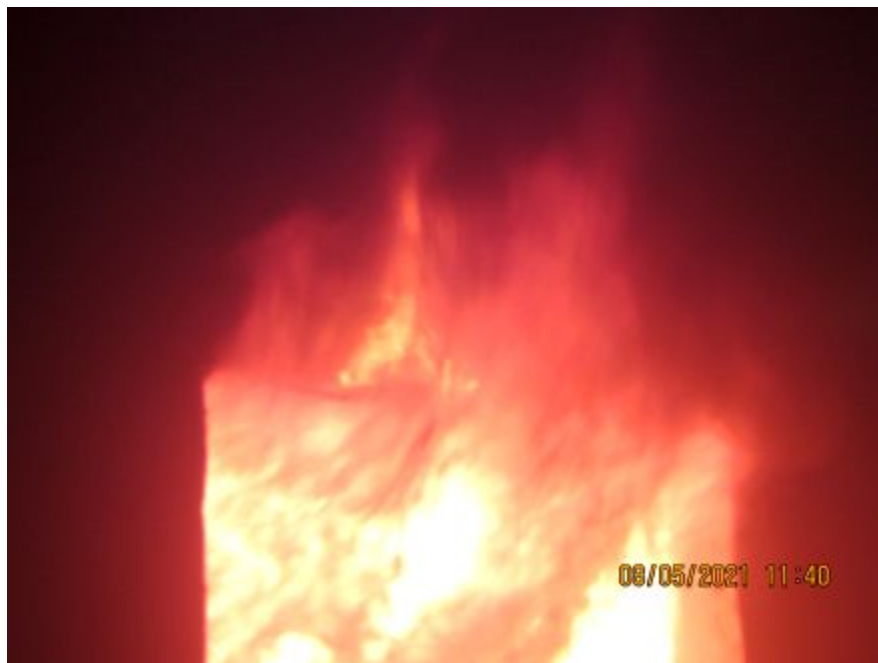
Photo No. 12 Flaming at window header
