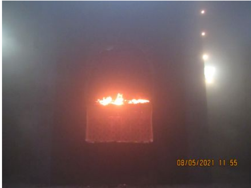
Photo No. 15 Gas off, residual flaming at header
