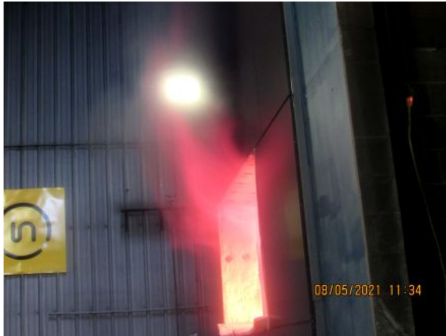
Photo No. 9 Flames exiting window opening
