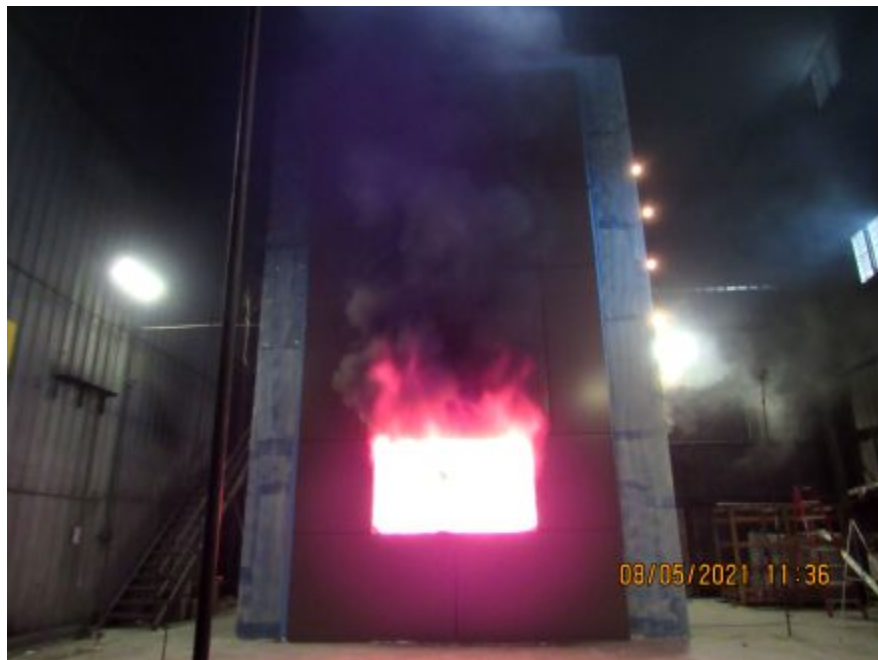
Photo No. 10 Flame tips at 1 meter
