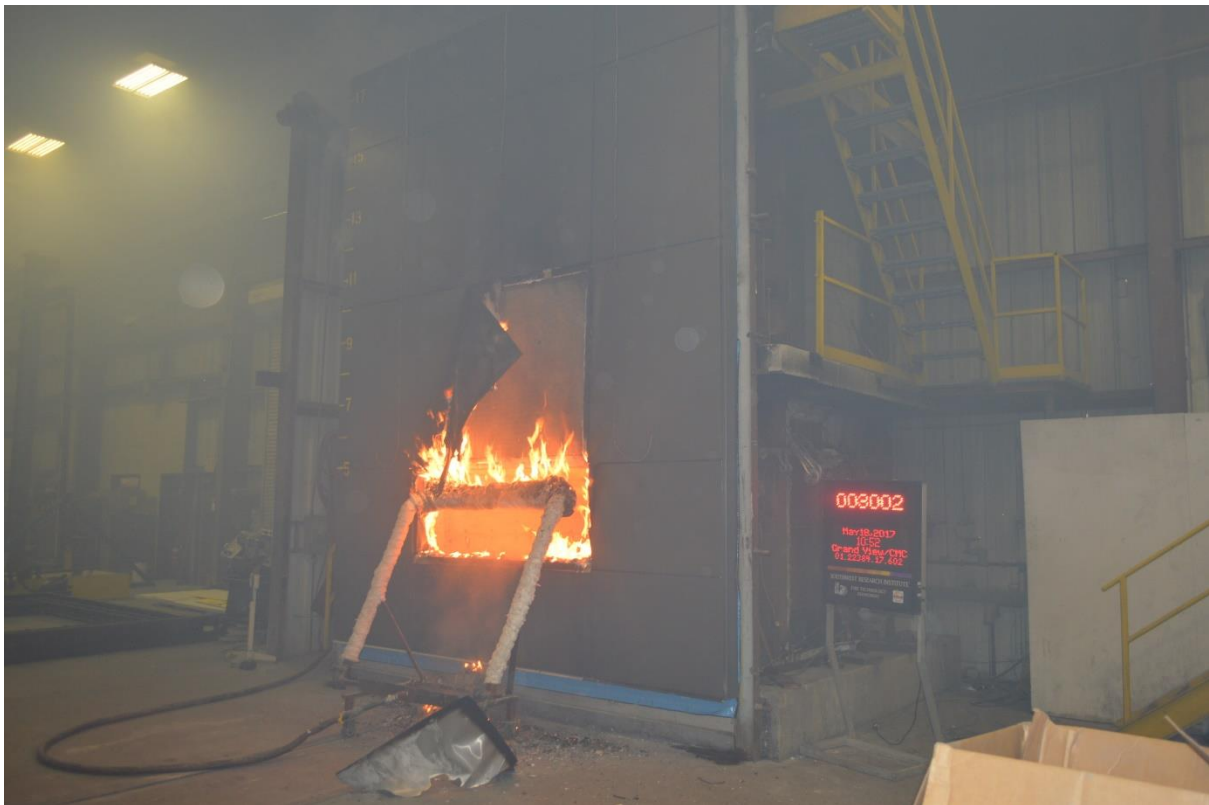
Figure B-15. Exterior View of Wall Assembly and Residual Flames after Burn Period.
