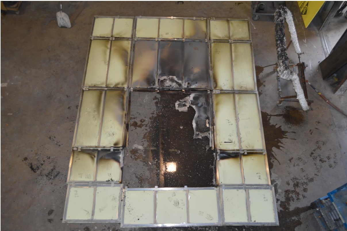
Figure B-19. Interior Face of Aluminum Composite Panels Posttest.
