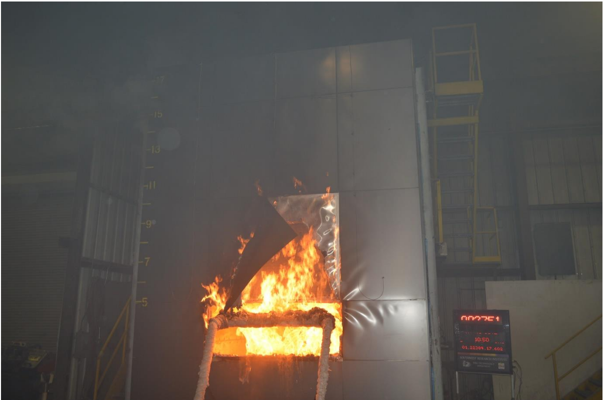
Figure B-14. Exterior View of Wall Assembly Approximately 27 min into Test.
