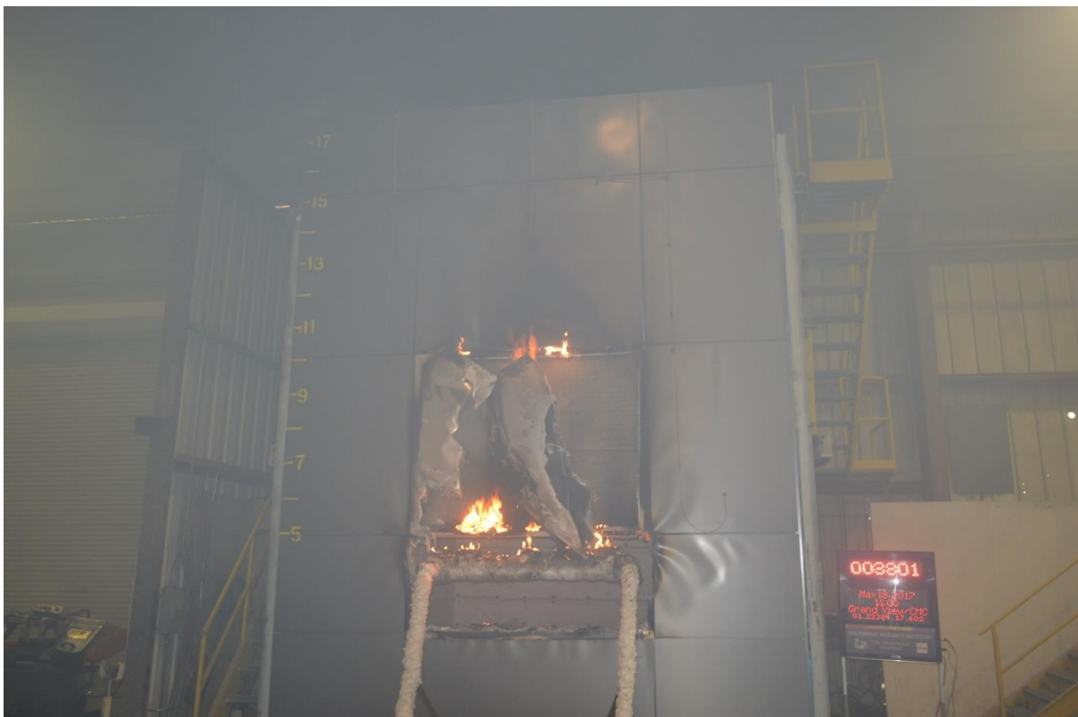
Figure B-16. Exterior Face of Wall Assembly 8 min after Burn Period.
