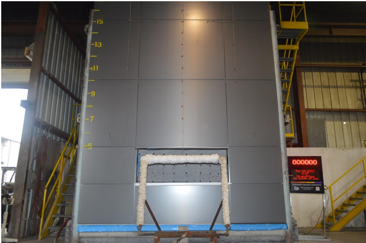
Figure B-5. Instrumented Exterior Face of Wall.
