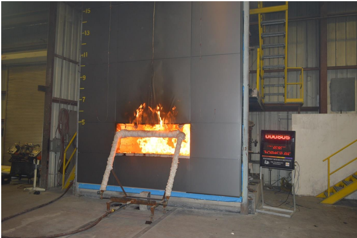
Figure B-9. Exterior View of Assembly 8 min 5 s into Test.
