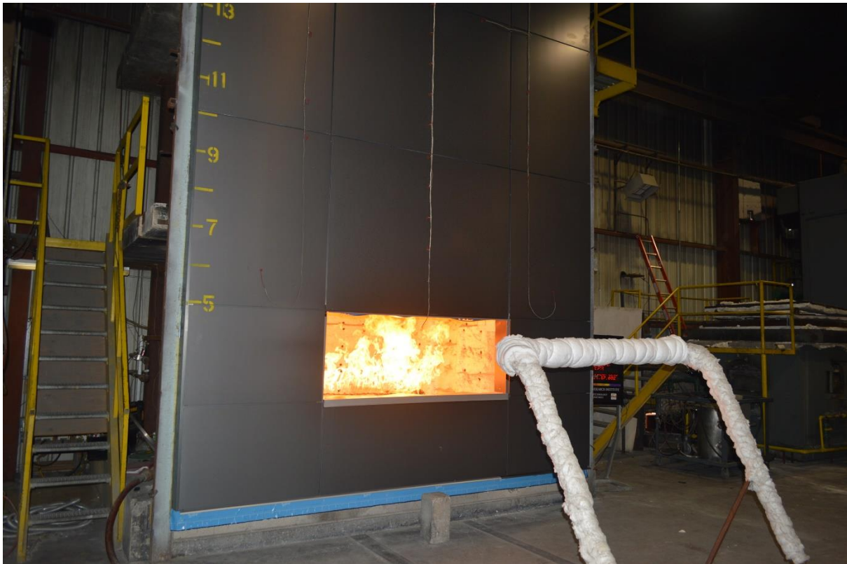
Figure B-7. Exterior View of Wall Assembly at Start of Test.
