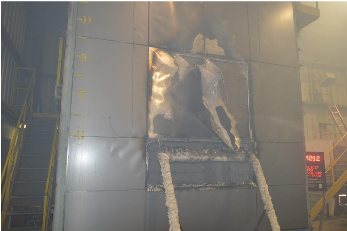
Figure B-17. Exterior Face of Wall Assembly immediately after Testing.
