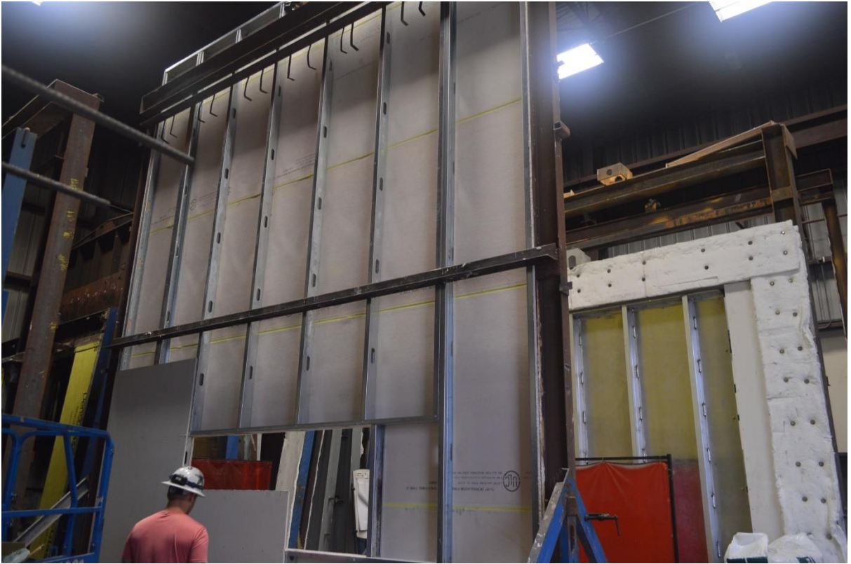
Figure B-1. Metal Stud Framing of Wall Assembly.
