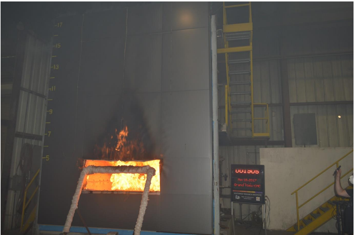
Figure B-12. Exterior View of Wall Assembly Approximately 19 min into Test.
