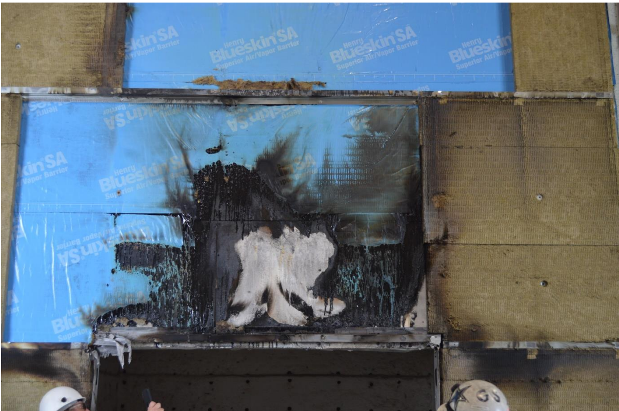
Figure B-20. Exterior View of Blueskin® SA Air and Vapor Barrier.
