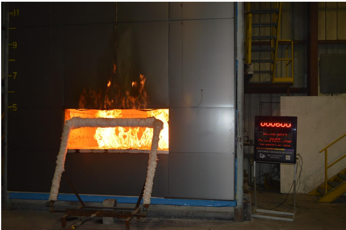
Figure B-8. Exterior View of Wall Assembly 6 min into Test.
