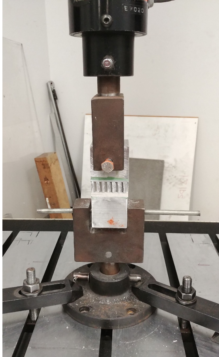
Photograph 1: Specimens were pulled in tension to failure.
