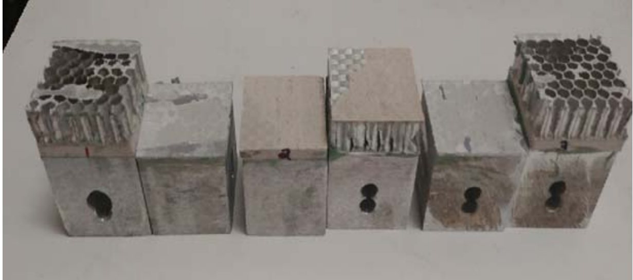
Photograph 2: Mode of failure Specimens 1,2,3.
