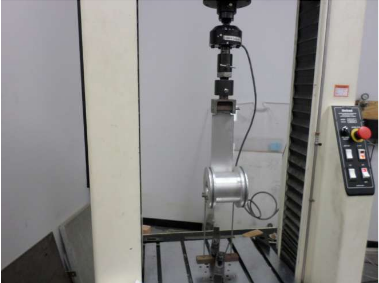
Photograph No.1 Climbing drum peel test set-up
