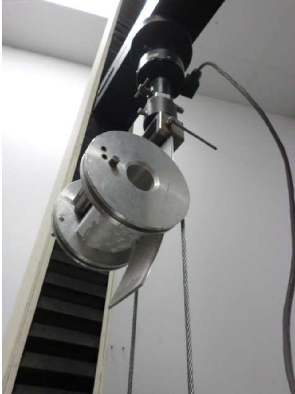
Photograph No.2 Climbing drum peel test typical mode of failure
