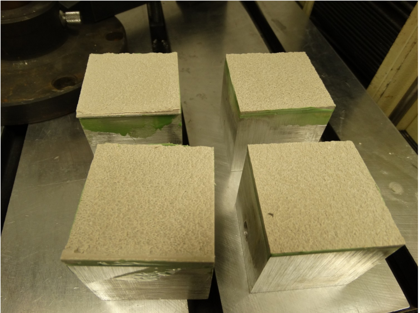
Photograph No 2: Typical Mode of Failure: Cohesive Failure Within the Specimen
